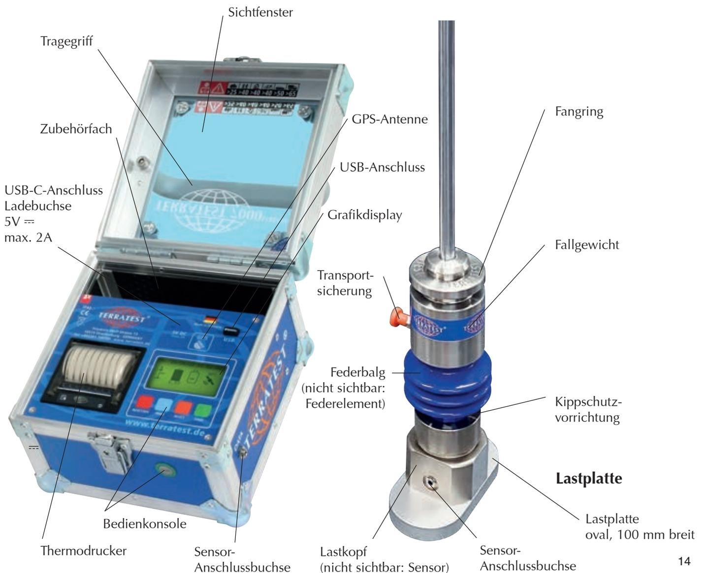
2.7 Ansicht Frontplatte Messcomputer TERRATEST 7000 STREAM / TERRATEST 7000 TRENCH
